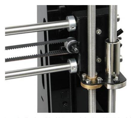
\*Note the direction of the driving wheel, the side with bolt head should be towards the A1, or it will scratch the acrylic plate.
