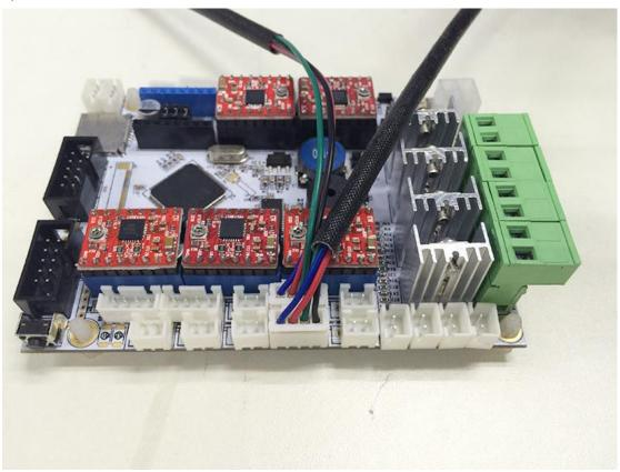
4) Connect Extruder motors. Connect extruder 0.
