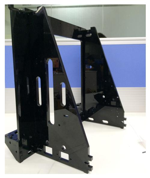
If the tab doesn't fit the hole, there must be some manufacturing faulty, please use the file to trim it.
