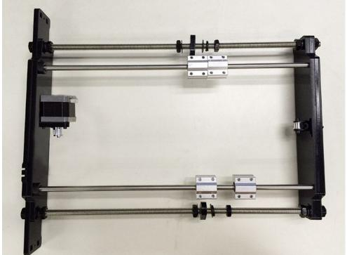
Look at this picture, the driving wheel and the pulley should be in a straight line.
