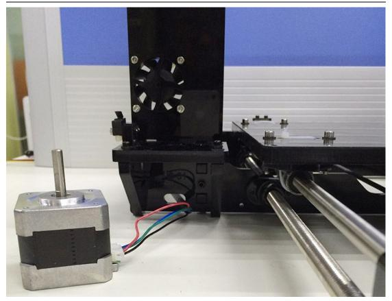
Step2.Screw up the motors on A5 with 4 M3 x 12 screws and M3 washers.
