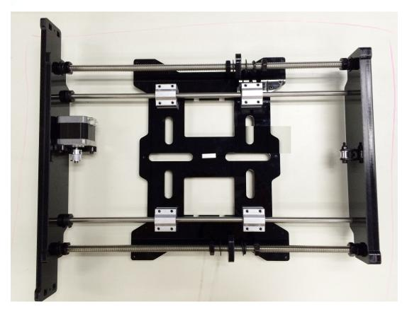
\* Note the direction of the building platform support, you can judge from the direction of the belt mount, whose direction is corresponding to the Y axis.
