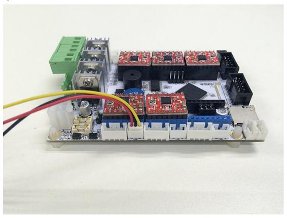
3) Connect fan for extruder 1, connect the other to FAN1.
