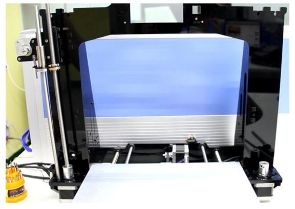
Step3. Thread the L470mm smooth rod into the X motor end > thread the extruder
