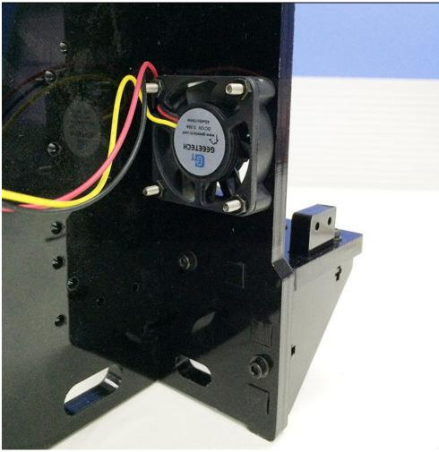
Note the direction of the fan, the side with wires is at outside. The fan is for the heat dissipation of the control board. You can see from the video.
