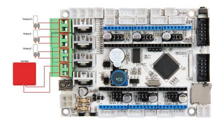
1) Connect heating wires for heatbed.
