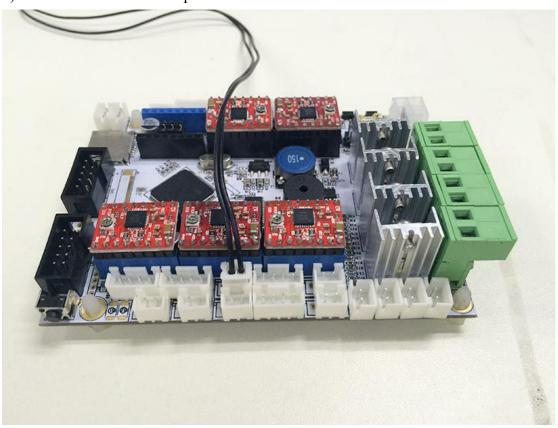
3) Connect wires for endstop of Z-axis at Z-Min.
