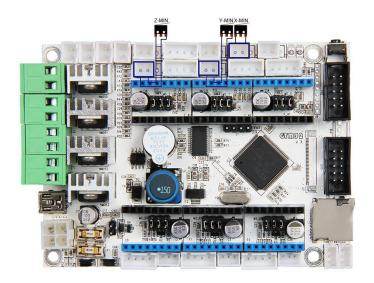
1) Connect wires for endstop of X-axis at X-Min.
