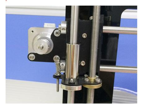
Step 4. Add another two locking rings on the smooth rod and thread the two X axis
