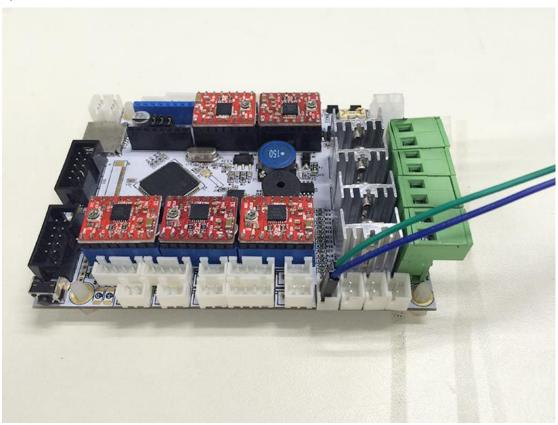
2) Connect wires for thermistor of hotend 1
