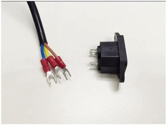
Step 2. Thread the wires that is connected to the red switch through another hole on the bottom of the right side panel(A2) from outside to inside and connect the 3 wires (brown, blue, yellow) to the socket, do not mix them up. Refer to the above picture. Then pull the other wires out.
