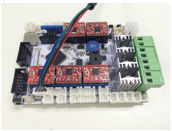
2) Connect wires for Y-axis motor.
