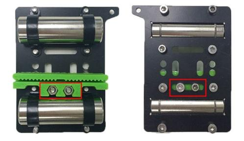
Step3. Fix the extruder holder on the front side of the X carriage using M4x6mm screws.
