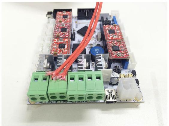
**Step3.** Connect wires for thermistor.
