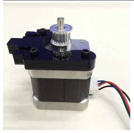
Step 3. Push the Y Motor holder tab into the square hole in Rear -Outside Plate and Rear - Inside Plate. You may need to use a little force, but be careful not to break or crack any of the Acrylic pieces. Secure the Y Motor holder with 2 M3x20 mm Screws, 2 M3 Washers and 2 M3 Square Nuts.
