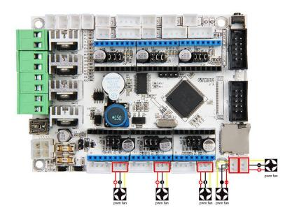
1) Connect fan for control board at FAN3.
