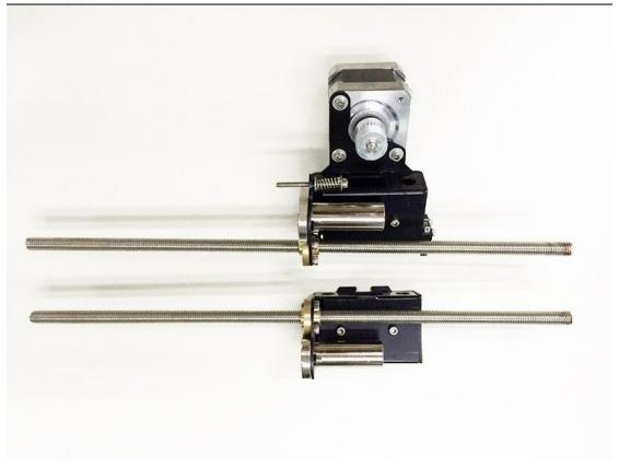
Step2. Plug the threaded rod on the X motor end to the left coupling on the left bottom of the Z axis. Then thread the 340mm smooth rod into the linear bearing.
