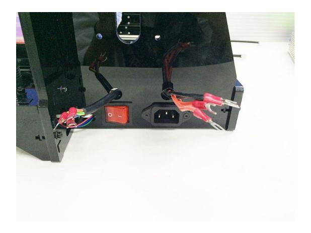
Step4. Mount the PSU on the right side panel with 3 M4  $\times$  12mm screws . And M4 washer.
