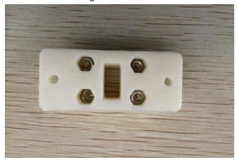
2. Loosely attach the two rectangular pieces to the main piece using four m3-16 screws. Make sure the flat surface is facing outward.
