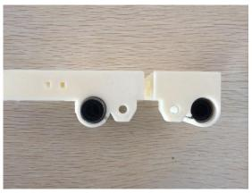
2. Insert the M5 nuts into the hexagonal slots on the X idler and the X motor holder. These two nuts must be tightly situated in the slots for proper z movement. If you find the two nuts falling out of place during z movement, heat the nuts on fire (do this carefully, of course) and insert hot M5 nuts into the hexagonal slots. The heat will melt the ABS a bit and provide a tight fit.
