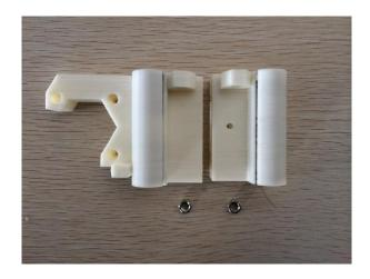
3. Use the M3-20 screw and nut to attach two 623zz bearing to the X idler.
