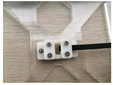
5. Wrap the GT2 timing belt around the Y motor's aluminum pulley, and around the 623zz bearings. Insert the other end of the GT2 timing belt into the Y belt holder and tighten the
