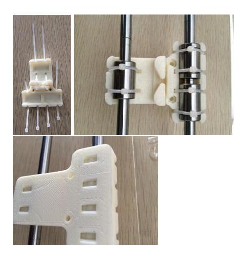
9. Wrap the GT2 timing belt around the X motor and the 623zz bearings. Tie both ends to the X carriage using zip ties. Make sure the belt is tight and there is no skipping when the carriage moves.
