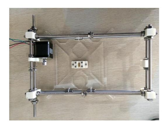
4. Attach the Y belt assembly to the acrylic bed using two m3-16 screws and two m3 nuts. Take 70cm of GT2 timing belt and insert one end into the Y belt holder. Tighten the two m3-16 screws to hold down the belt.
